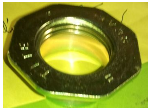
Bad sample (Milling moke is detected by camera)
