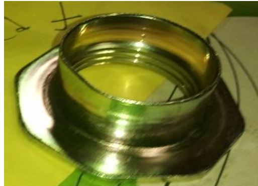
Bad Sample (with bend is not detected by camera)
