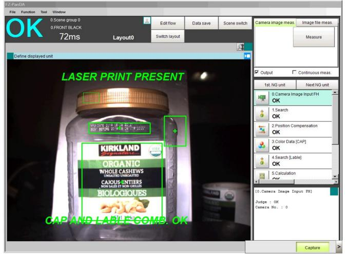
The below figure shows that the cap matches the sticker and all the conditions including laser marking are ok and hence the sample is OK
