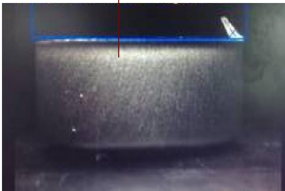
Flash Defects. (Side Camera.)
